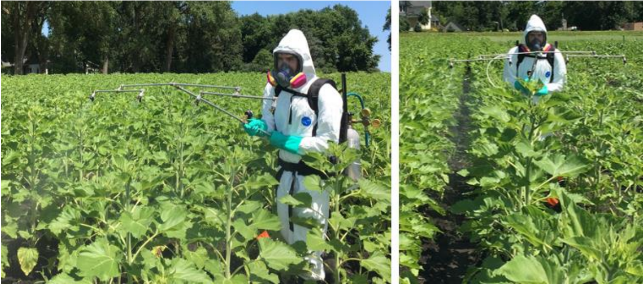
Figure 1. CO 2 powered backpack sprayer equipped with a 1.5 meter boom
