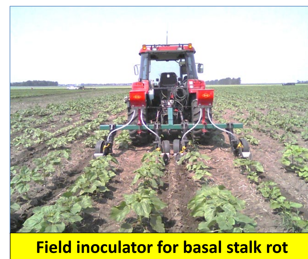
Field inoculator for basal stalk rot
