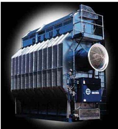
**Figure 124. A high temperature column dryer used for drying sunflower. (K. Hellevang)**
