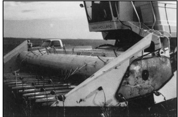
■ Figure 122. Rotating drum with metal projections. (V. Hofman)
