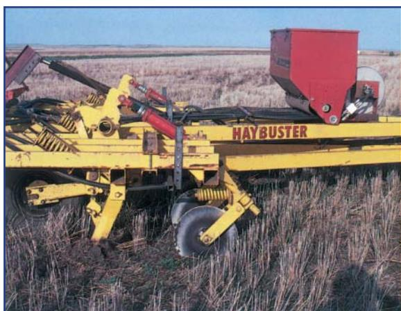
■ **Figure 11. Undercutter sweep machine used to prepare seedbed, control small weeds and conserves soil moisture.** (Al Black)
