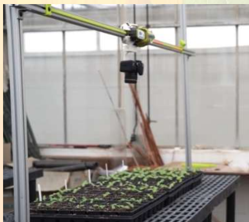
Fig. 2. Dronwer 2.0 RGB imaging platform. A downward-facing RGB camera mounted on the Dronwer 2.0 gantry captured time-series images of sunflower trays at fixed positions. Imaging and video capture were conducted regularly for 28 days post-inoculation to monitor BSR wilting, whole-plant desiccation, and mortality for image based scoring.
