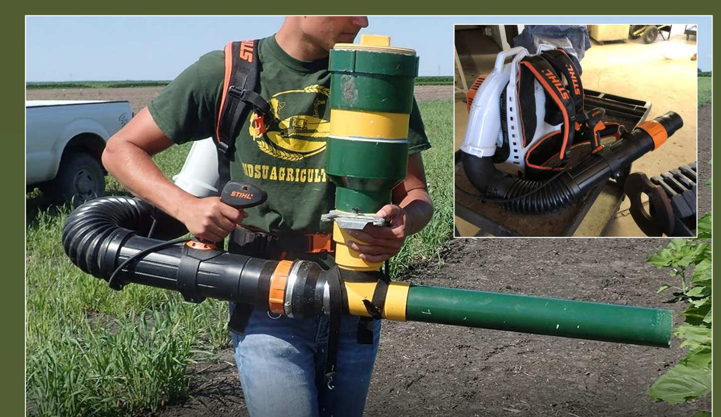
Figure 1. PVC attachment connected to a backpack leaf blower. The leaf blower creates airflow for a hailing medium (field pea seed) to gain enough force to cause damage to leaf and stem tissue but avoiding lodging issues.
