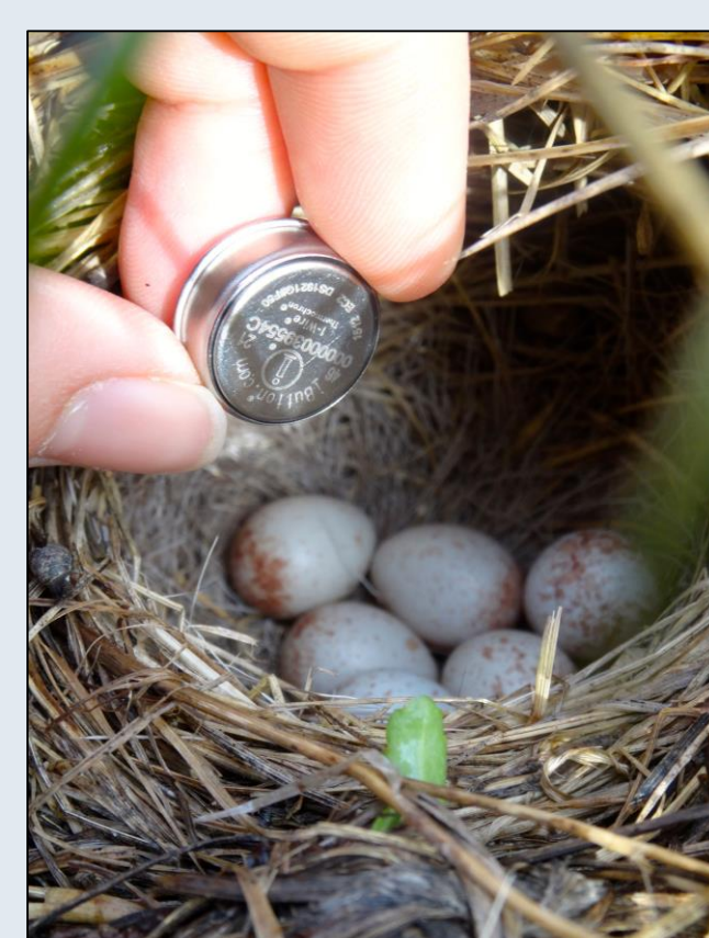
Figure 4. iButton sensors can be hidden in nests to wirelessly monitor incubation behavior of female blackbirds by recording the time and temperature of a nest every 3 minutes. This data is from a dark-eyed junco ( Junco hyemalis ) nest [3] .
